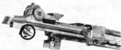
Figure 10. Position of the selector for removing the connector assembly (rifle modified for selective firing).
